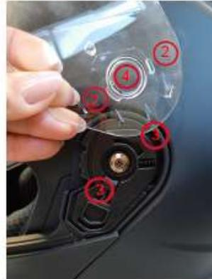
**Dismantling:** Lift the outer visor in open position. Pull backwards the visor lock (1). Pull the visor outwards and extract it. Repeat on the other side.
